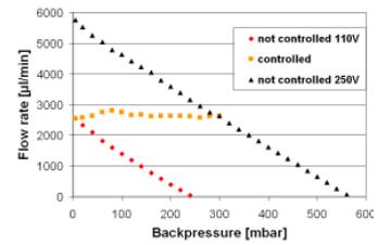
Fig. 4 First performance graph of piezo sensor controlled pump
