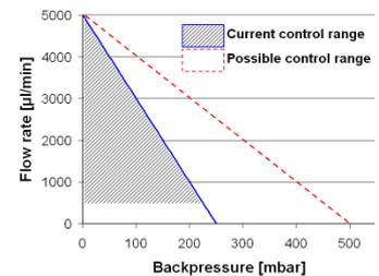
Fig. 5 Controllable flow range of piezo sensor
