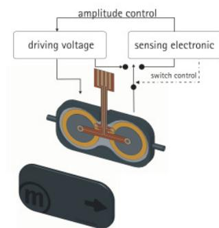
Fig. 3 Flow-sensing schematic of intrinsic sensor function
