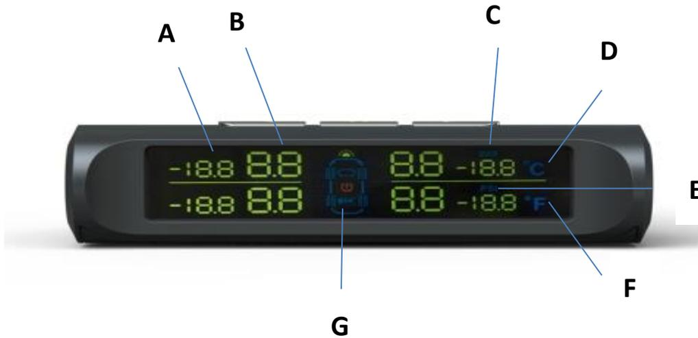
A、 current tire temperature value    B、 current tire pressure value    C、 pressure unit
