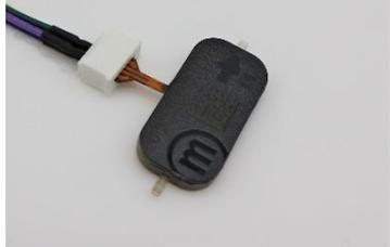
The three figures on the right illustrate how to **connect the micropump to the plug**. The pump cable has to be inserted with the contact surfaces orientated down into the plug. Both components are firmly connected by closing the white plug. When **disconnecting** the pump, the board connector must first be opened! Verify yourself that the board connector is always locked before start running the pump. Otherwise, this will lead to a malfunction of the pump or the electronics.
