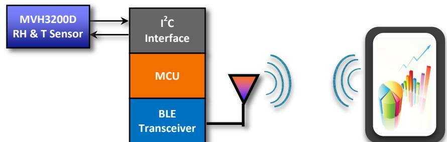
Sensing module functional diagram
