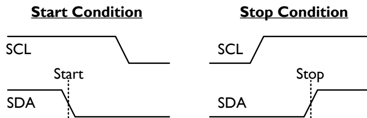
Fig. 8: I^2C bus start and stop conditions.
